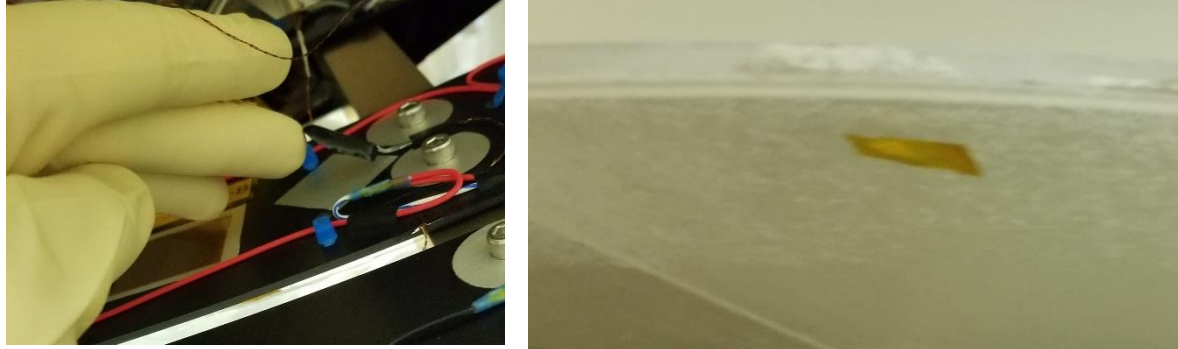
Figure 15: At left is a sensor that was attached to an aluminum control zone with stycast, and at right is a piece of Kapton tape which originally had a sensor under it.
