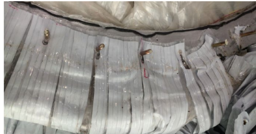
Post-flight end fitting inspection showing elongated holes.
