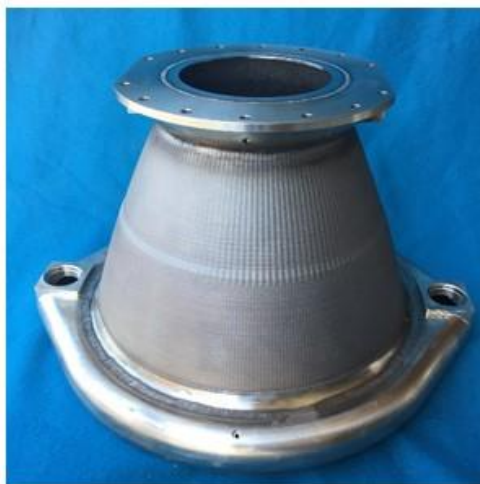
GTAW of Aft manifold
