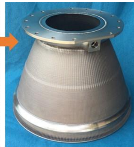
EB Welding Forward Manifold
