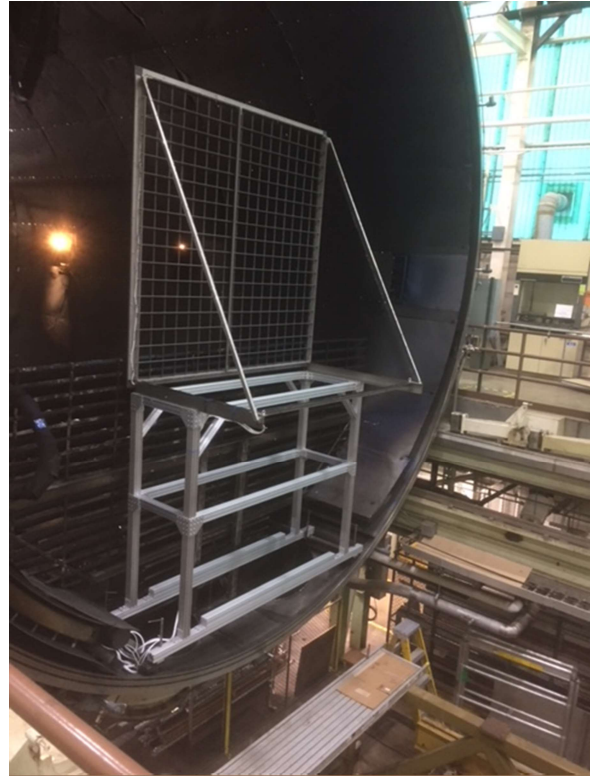
Figure 4 A picture of the thrust vector probe located at the downstream end of VF 6
