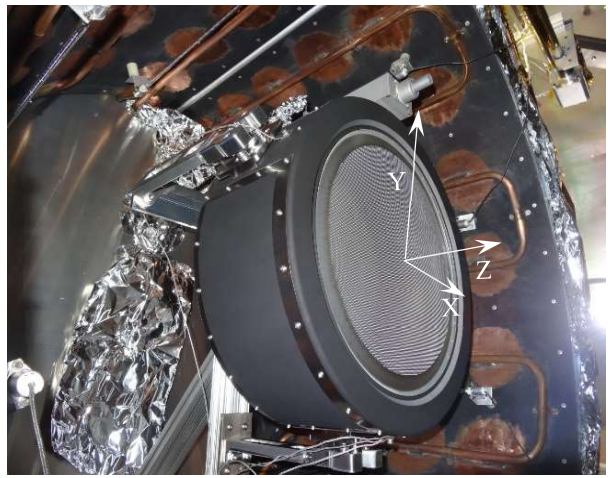
Figure 5 Pictures of the flight NEXT-C thruster mounted within the thermal shroud used to perform the TVAC testing.
