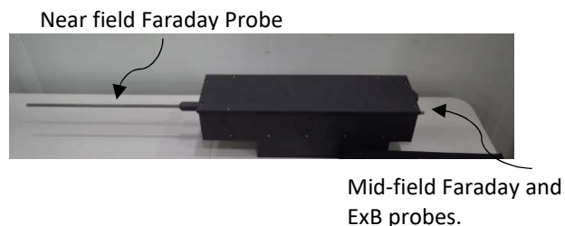
Figure 3 A picture of the Mid-field probe suite containing the probes used to make the ion beam measurements.
