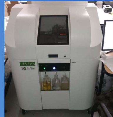
UTEP ExONE M-lab Binder Jet AM machine
