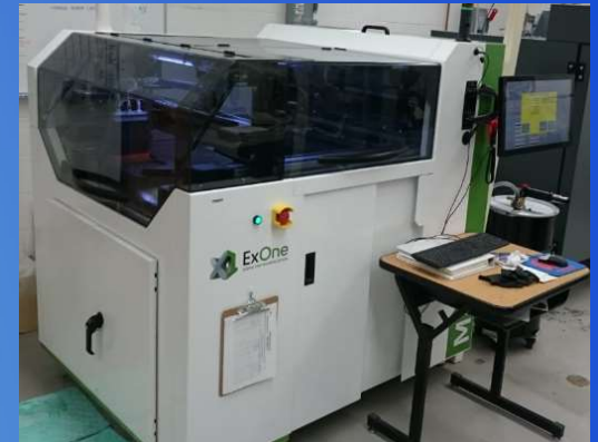
UTEP ExONE M-Flex Binder Jet AM machine
