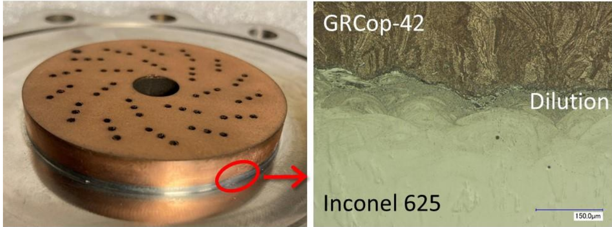
Figure 19. Bimetallic L-PBF Injector face using GRCop-42/Inconel 625 and the interface diffusion between these alloys.
