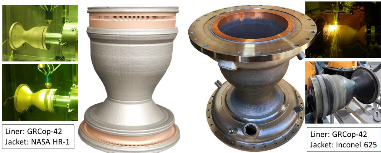
Figure 20. Bimetallic Jacket using LP-DED Process. (Left) GRCop-42 L-PBF liner cladded at RPMI with NASA HR-1 Jacket using an interface alloy; (Right) GRCop-42 L-PBF liner cladded at DM3D with Inconel 625 Jacket.
