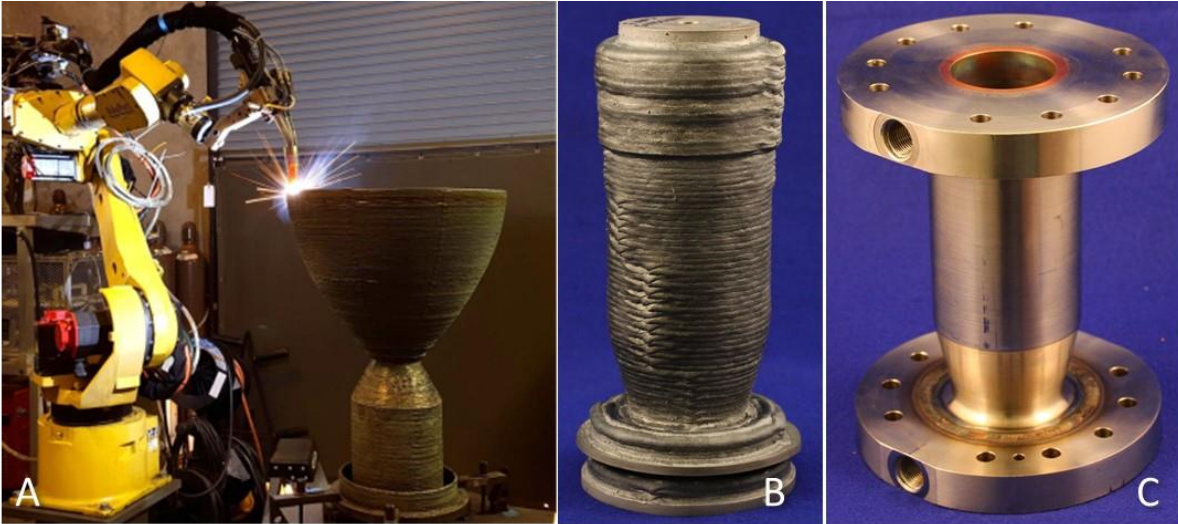
Figure 10. Arc Wire DED (AW-DED) process. A) Process demonstration of monolithic chamber, B) Inconel 625 jacket applied to GRCop-84 L-PBF liner, C) Finished bimetallic chamber using AW-DED jacket.
