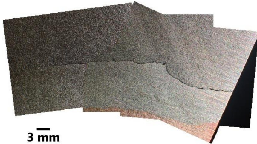
Figure 12. Macro photograph of crack in Inconel Alloy 625/GRCop-42 sample used for interface bond strength testing of EBW-DED. Crack is between the first and second Inconel Alloy layers.
