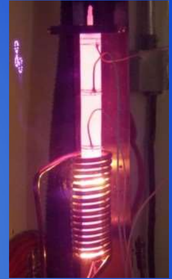
TZM Mo-alloy heat pipe. Courtesy Advanced Cooling Technologies.
