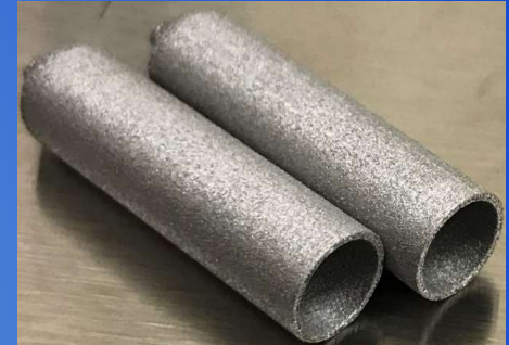
As-built L-PBF AM W leak test specimens with 0.5 mm wall thickness.
