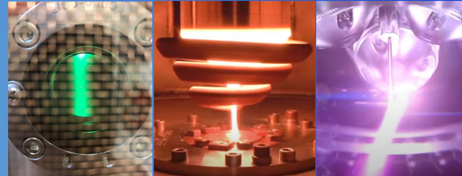
MSFC Tekna Tek15 plasma spheroidization of W powder.
