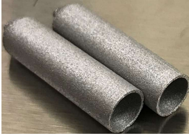
Fig 7. As-built L-PBF AM W leak test specimens with 0.5 mm wall thickness.
