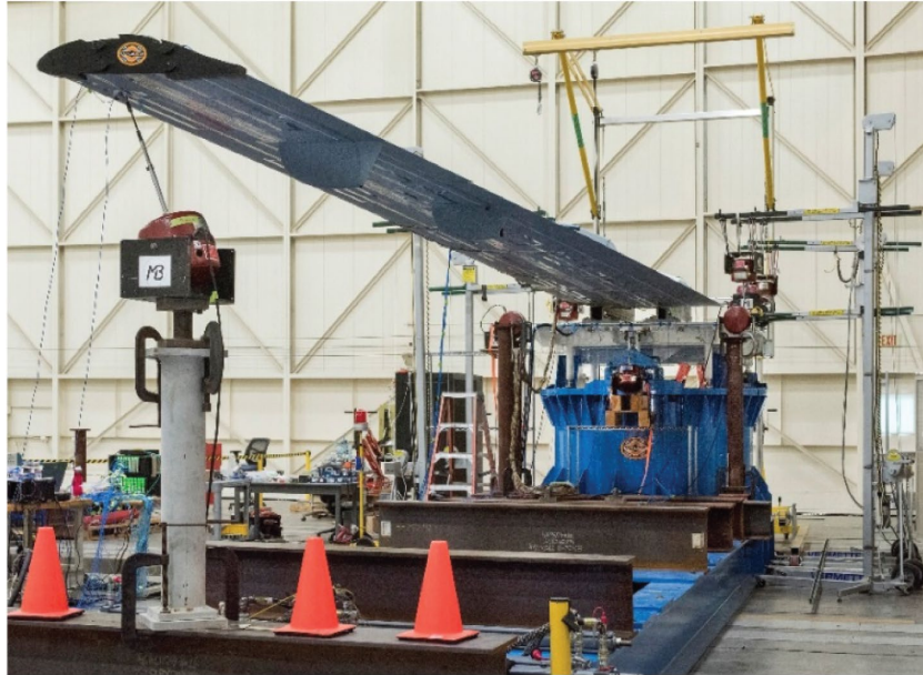
Figure 12. The CReW wingtip shaker.
