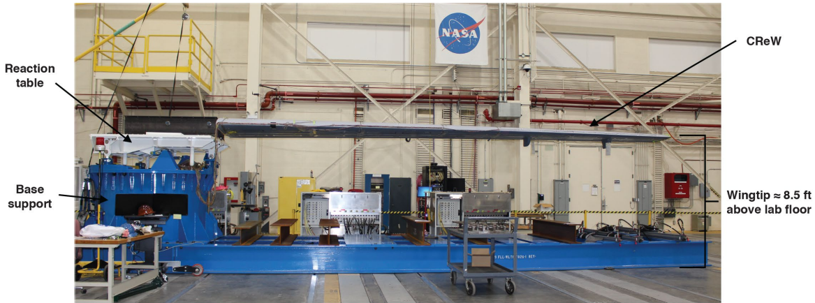
Figure 6. The modal test setup with the CReW mounted on the WLTF with wingtip approximately 8.5 ft above the floor of the FLL.
