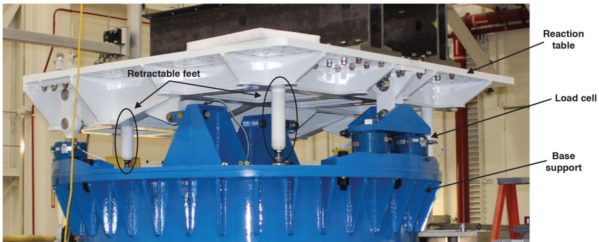
Figure 4. The WLTF reaction table supported with four retractable feet (two shown) and seven load cells (four shown).
