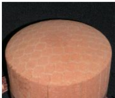
AVCO 5026-39 HCG (Filled Epoxy Novalac in Fiberglass-Phenolic Honeycomb) Now manufactured by Textron
