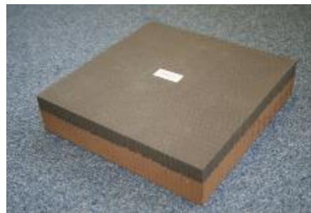
Graded Ablator High Density to Lower Density
