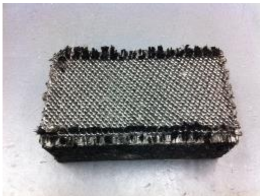
3-D Woven Carbon Fibers Infiltrated with Resin
