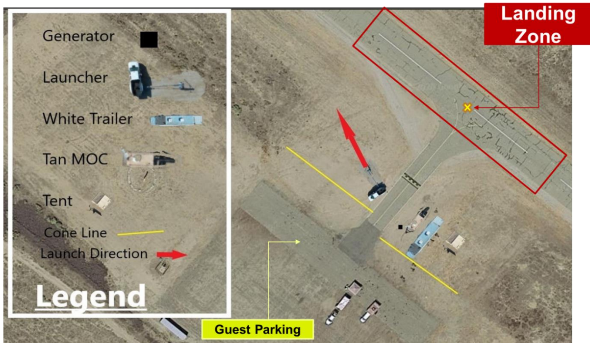
Figure 3-1. NASA SIO Ground Layout
