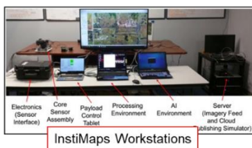
Figure 3-2. AiRanger fielded system components
