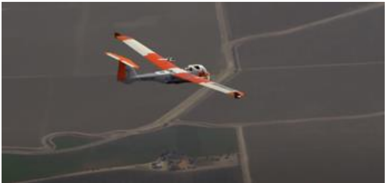
Figure 2-12. AiRanger enhanced visibility features
