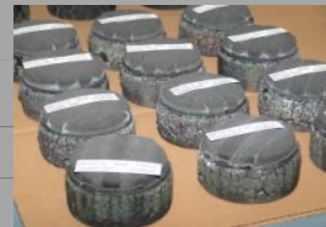
Arcjet ablator coupons, post test
