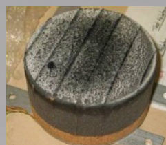
Tested Solar tower ablator coupon
