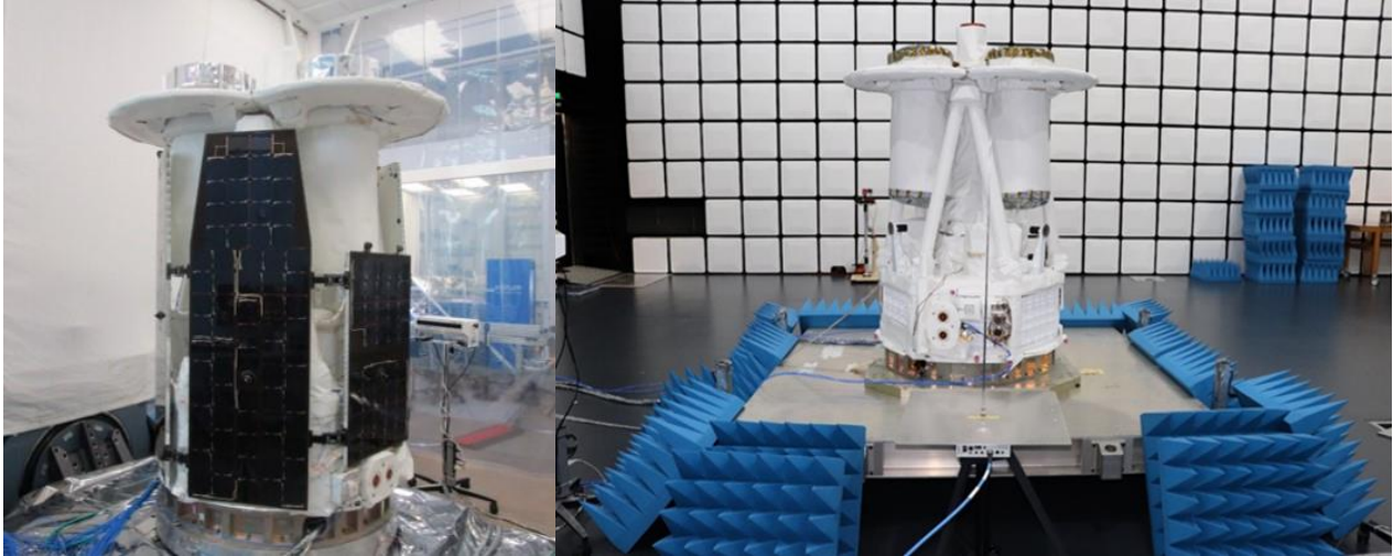
Figure 10: IXPE observatory on vibration table (left) and being prepared for acoustic testing (right)
