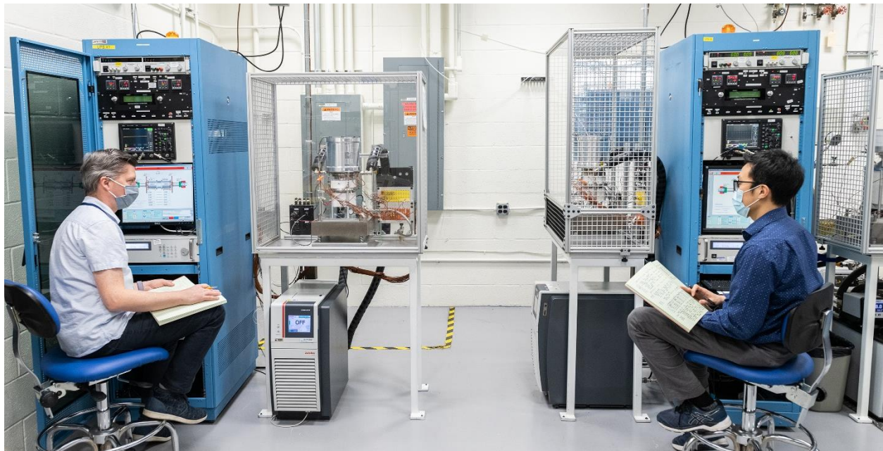
Figure 1. Engineers in the Stirling Research Laboratory at NASA's Glenn Research Center monitor Stirling Convertors on continuous test for the Dynamic Radioisotope Power Systems (DRPS) Project. Credit: NASA.
