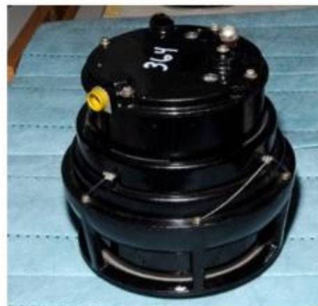
Figure 4.11. Cabin pressure regulator cross-section (top) and in exterior view (bottom).
