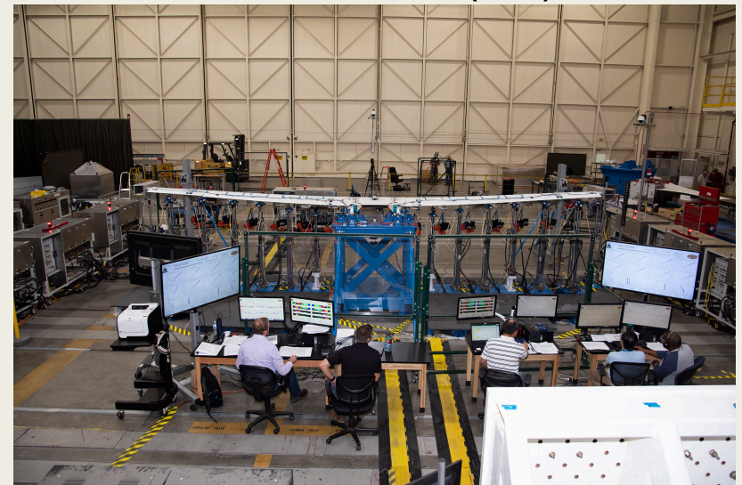
Ground Vibration Test (GVT)
