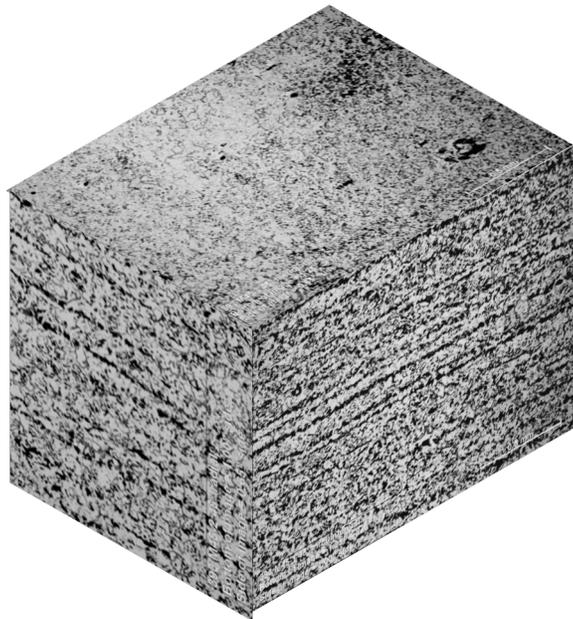
Figure 7.2.1.2-12: Micrographs of PV0296 CP-279 at 45 Degree Location, 50X
