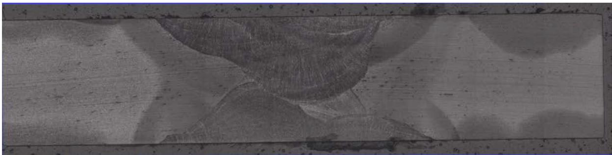
Figure 7.5.2.2-2: MV50466-8 Inner Weld Macro
