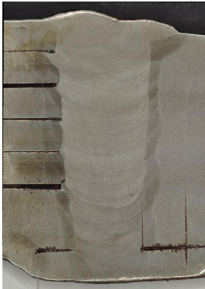
Figure 7.5.3.2-4: V0032 Head-to-Shell Weld Macro
