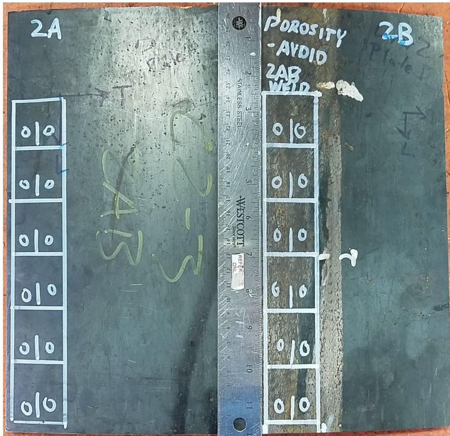
Figure 7.5.1.3.4-1: Specimen Cut Plan da/dN V0023 Seam Weld
