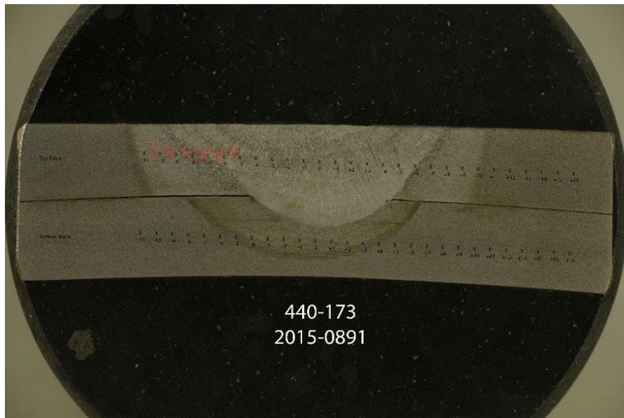
Figure 7.5.1.2-7: MV50466-8 Seam Weld 440-173 Indent Locations
