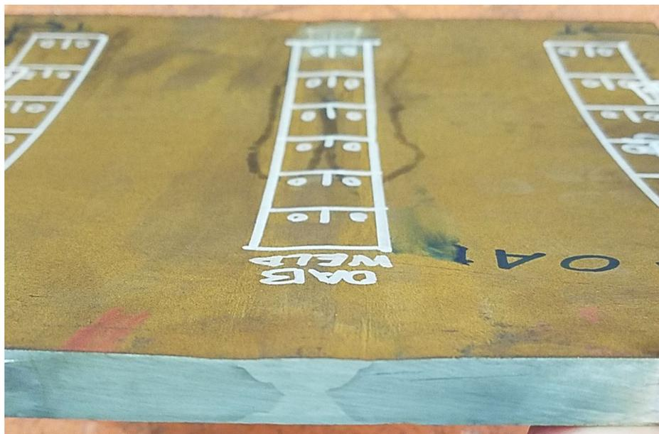
Figure 7.5.2.3.4-2: Specimen Cut Plan da/dN V0023 Inner Layer Weld (Continued)
