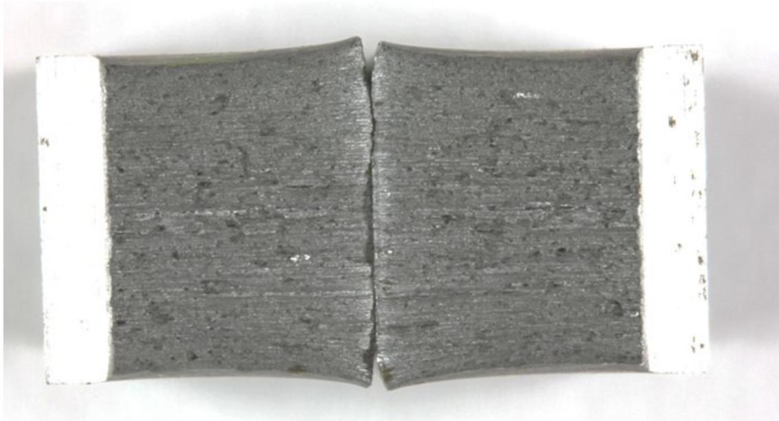
Figure 7.3.2.3.5-2: V0125 1143 V-Notch Charpy Fracture Surface 74°F
