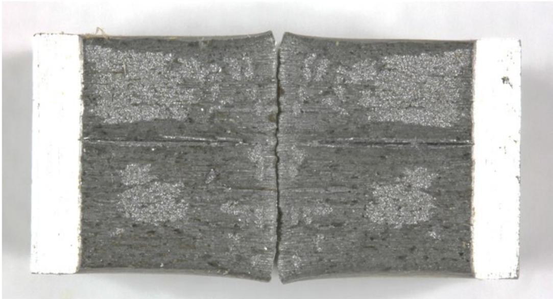
Figure 7.3.2.3.5-3: V0125 1143 V-Notch Charpy Fracture Surface -40°F
