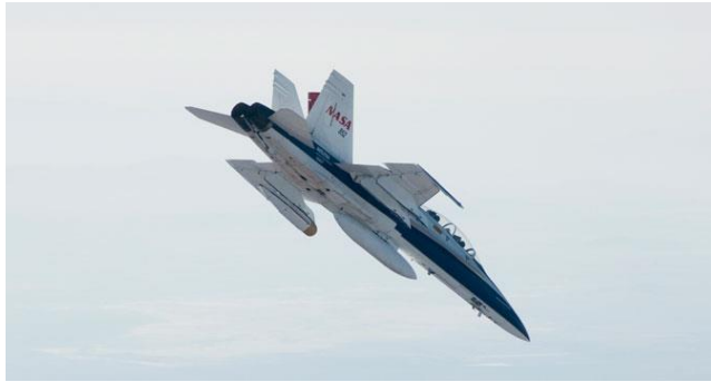
NASA Armstrong F-18 Testing Mars Science Laboratory (MSL) Landing Radar
