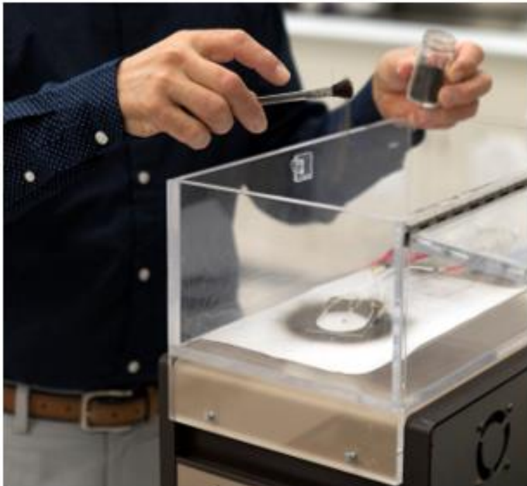
Testing of a transparent EDS which uses dynamic electric fields to remove dust from surfaces
