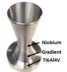
Gradient alloy rocket nozzle
