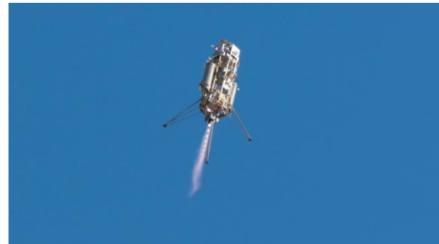
Flight Opportunities Program Masten Xombie Testing Vision Landing System (VLS) for Perseverance Mars Rover
