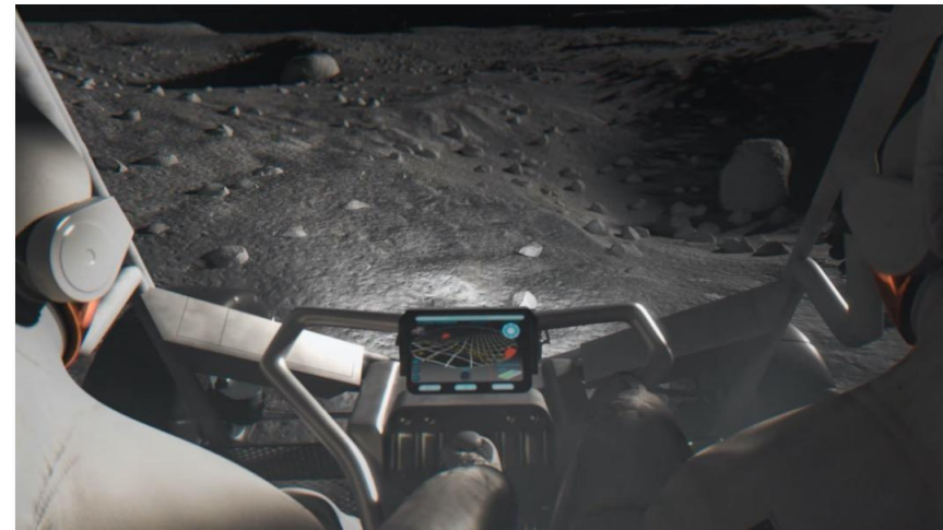
Artist rendition of LTV using 3-D Imaging flash LiDAR terrain mapping
