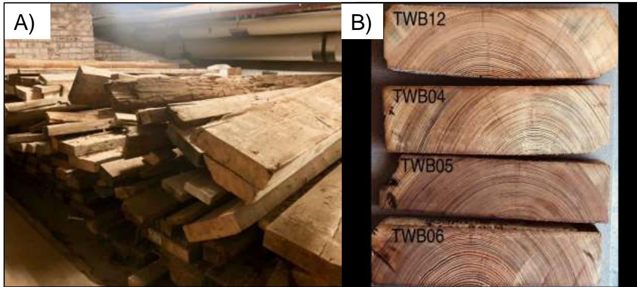
132 Figure 2: A) Remnant longleaf pine joists stored in the basement of the Terminal Warehouse in 133 Chelsea, New York City; B) Four joist timbers (TWB04, TWB05, TWB06, and TWB12) after 134 being cut, sanded, and prepared for dendrochronological analysis.
