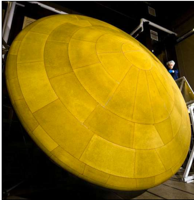
Phenolic-Impregnated Carbon Ablator (PICA) Mars Science Laboratory, Mars 2020
