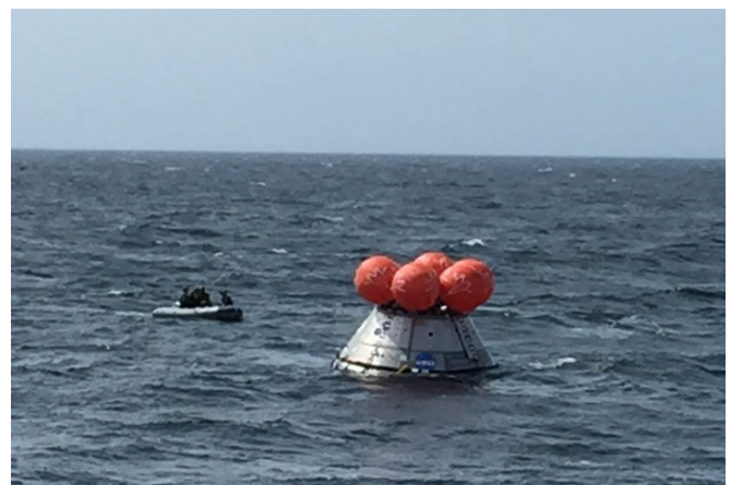
Fig. 1. Orion CM with CMUS bags after uprighting testing.
