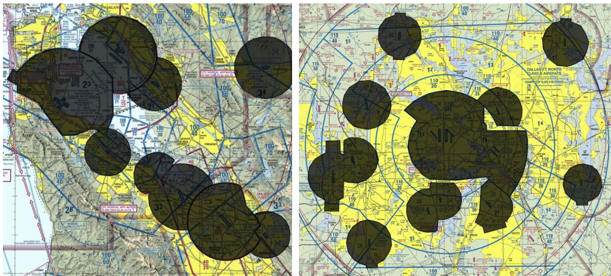
Figure 10: San Francisco Bay Area [900 nm 2 ] (left) and Dallas Fort Worth [2500 nm 2 ] (right) airspace top view. Dark shaded areas represent core (to the surface) airspace which require a clearance and communication to operate within them. San Francisco top view is approximately 30 by 30 nautical miles (900 nm 2 ). Dallas Fort Worth is approximately 50 by 50 nautical miles (2500 nm 2 )
