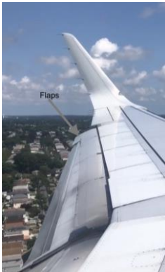
Figure 2: Flaps on Airbus A321
