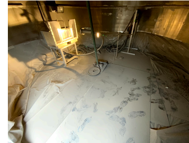
BP-1 dust coating over entire 15-foot vacuum chamber after pump-down outgassing
