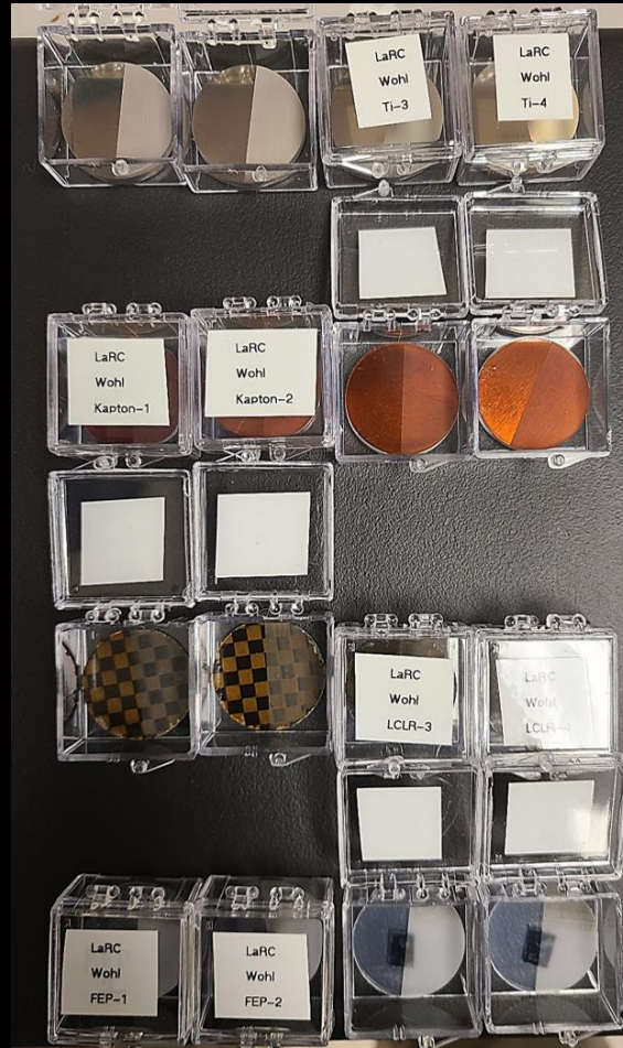
Laser Ablation Patterning on half of metal and polymer flight sample coupons
