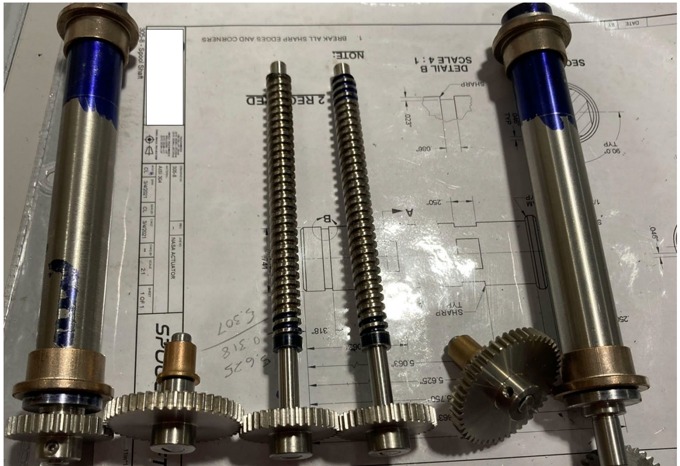
Fig 11 Spooling assembly shafts with bushings and gears
