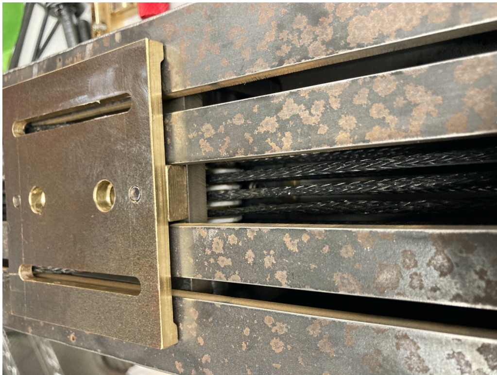
Fig 14 Center carriage running in the inner sleeve
