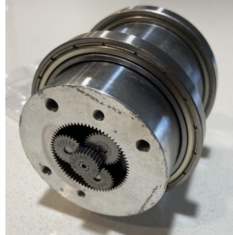
Figure 19: Inner Hub with Bearings and Gearset
