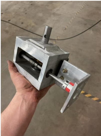
Figure 46: Manufactured Motor Mount Steering Assembly Manufacturing:
