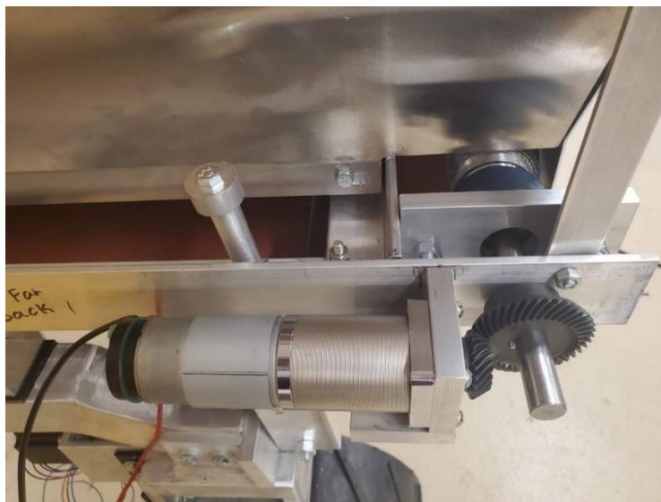
Figure 57, DC motor and gears to drive hopper conveyor.
