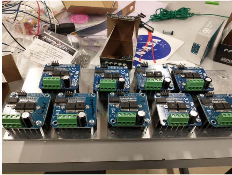
Figure 60, Mounting BTS motor controllers to plate
