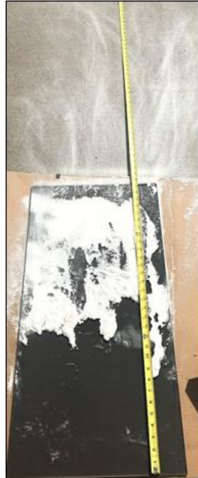
Figure 17: Dust Removal on Glass Pane
