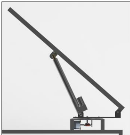
Figure 2: Solar Panel CAD, Side View
