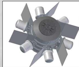
Example DRPS concept images based on Stirling conversion (6 converters per generator shown)
