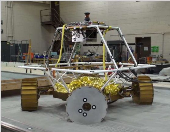
All Wheels Rotated to 45 Degrees
