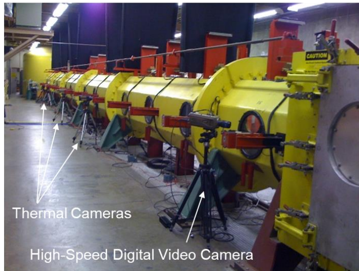
Exterior of the Test Section
