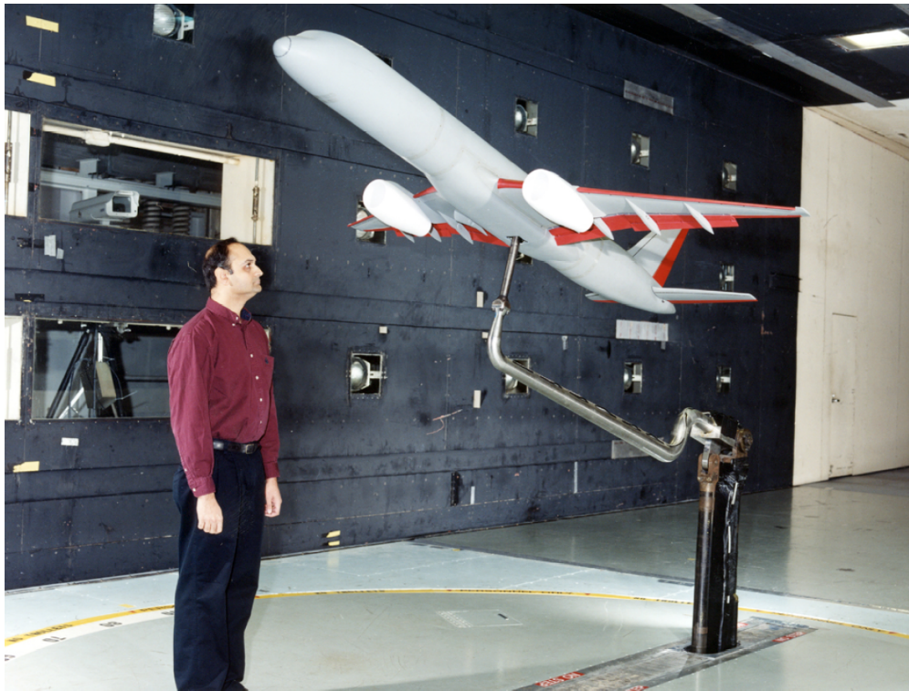
Figure 4: GTM wind tunnel test article installed in the NASA Langley Research Center 14×22 Ft Subsonic Tunnel (credit: NASA Langley Research Center).
