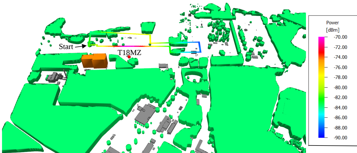
Figure 1. Received control signal power shown as a colored line along a flight path over the CERTAIN I Range at Langley Research Center, assuming a receiver gain of 2 dBi. The transmitter for the T18MZ controller is situated at the red dot.
