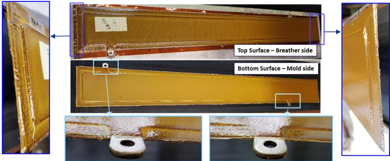
Fig. 17 Photographs of a completed conductor with 17X MMEI for GRC bus bar prototype showing high quality finish
