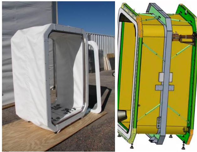
Fig. 7 Active-Active Mating Adapter Prototype at Desert Field Test and CAD Image of Mechanisms
