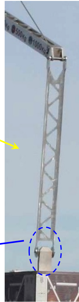
Lifting links used to provide structurally stiff connection to payload
