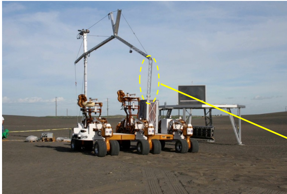
Precision placement of payloads on Chariot mobile base
