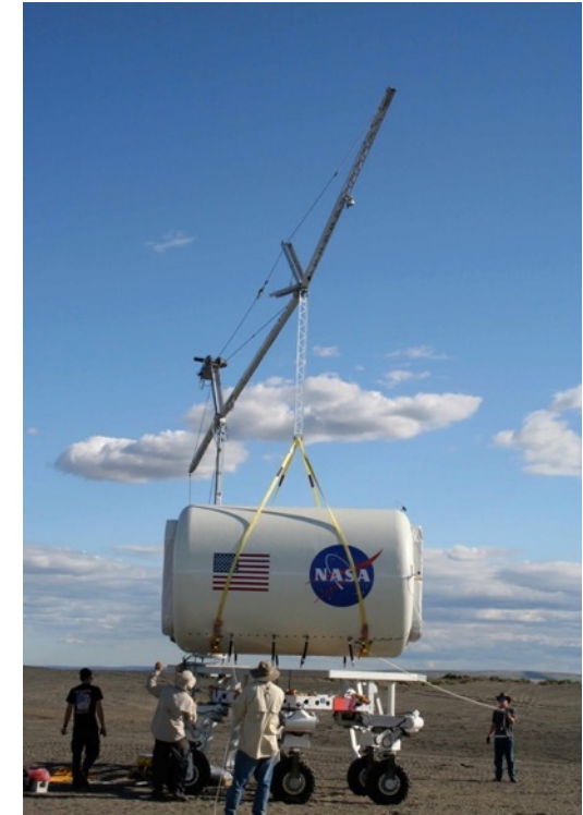
Versatility for unplanned operations: here shown field adapted for large payload handling of simulated habitation modules
