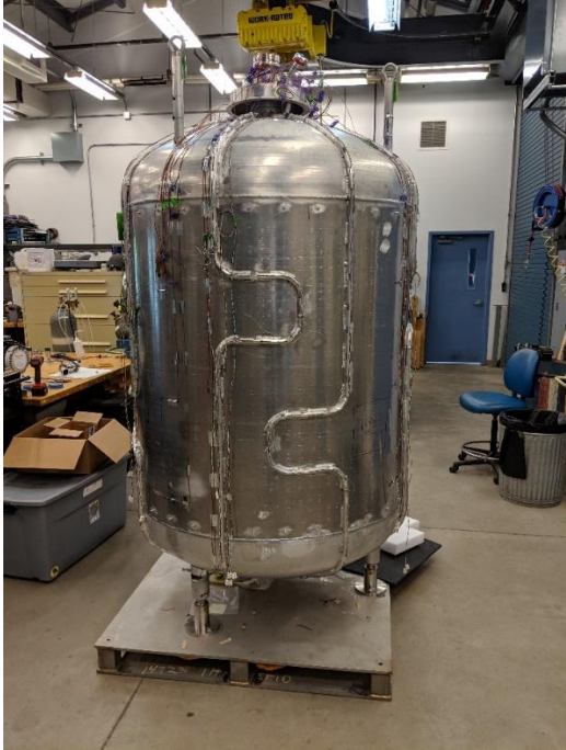
Figure 3: Tank with tubes welded to the tank wall. Credit NASA.
