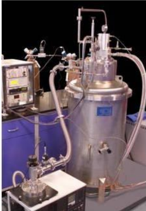
Figure 1: Cryocooler mounted on top of a tank. Credit NASA.
