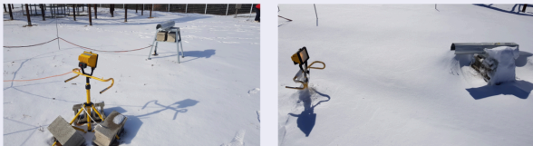
Fig. 1. Photos of the PIP setup during the 2018 ICE-POP field campaign in South Korea that coincided with the Winter Olympics. PIP is composed of a camera, which is shielded by a visor in the pictured setup, and a lamp, which is used to back light the precipitation particles.
