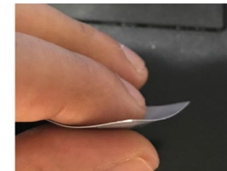
Flexible, printed supercapacitor for energy storage
