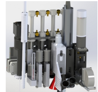
Figure 3. Next-generation tool heads for printing and processing of a wide range of printed electronics and sensors.
