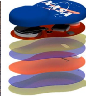
AstroSense wireless wearable sensor (cortisol, temp, humidity)
