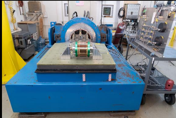
Fuel Cell Stack installed on the Vibration Table at JSC
