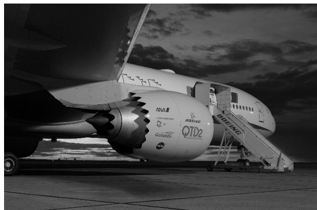
FIG. 20. A photograph showing a chevron nozzle tested on the Quiet Technology Demonstrator 2 (QTD2) (courtesy Boeing Aerospace Company). run of sustained research for noise, and support was waning. In 2006, new management for
