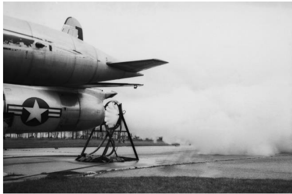
FIG. 9. A water-injection noise reduction concept investigated at NACA. Reprinted with permission from M. C. Kurbjun, NACA-RM-L57L05, National Advisory Committee for Aeronautics, Washington, DC (1958) (Ref. 33).
