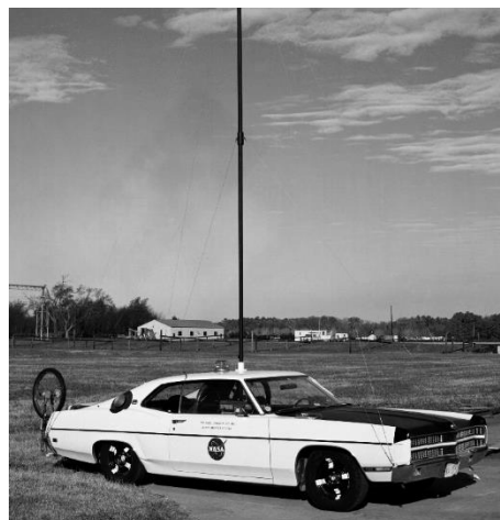
FIG. 15. A setup used to investigate the effects of forward flight on jet noise radiation. Reprinted with permission from T. D. Norum, NASA-TP-1326, National Aeronautics and Space Administration, Washington, DC (1978) (Ref. 86).
