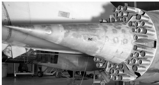
FIG. 24. A tube suppressor tested during the SCR program. Reprinted with permission from R. R. Burley and V. L. Head, NASA-TM-X-2919, National Aeronautics and Space Administration, Washington, DC (1974) (Ref. 165).
