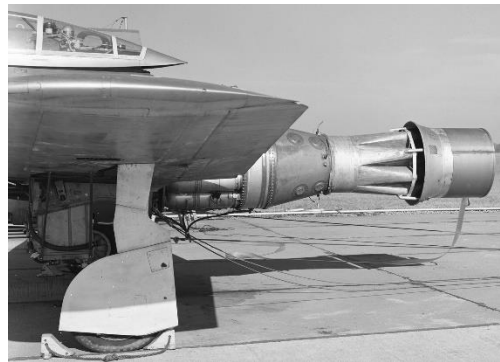
FIG. 6. A mixer-ejector concept tested at NACA. Reprinted with permission from W. D. Coles, J. A. Mihalow, and E. E. August, NACA-TN-4317, National Advisory Committee for Aeronautics, Washington, DC (1958) (Ref. 30).
