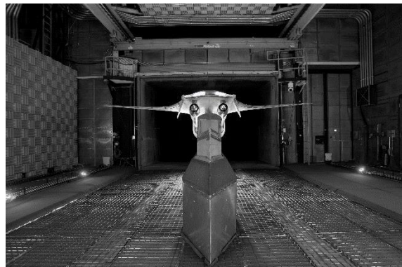
FIG. 21. The hybrid wing scale model in the 14 x 22 tunnel at NASA Langley Research Center.
