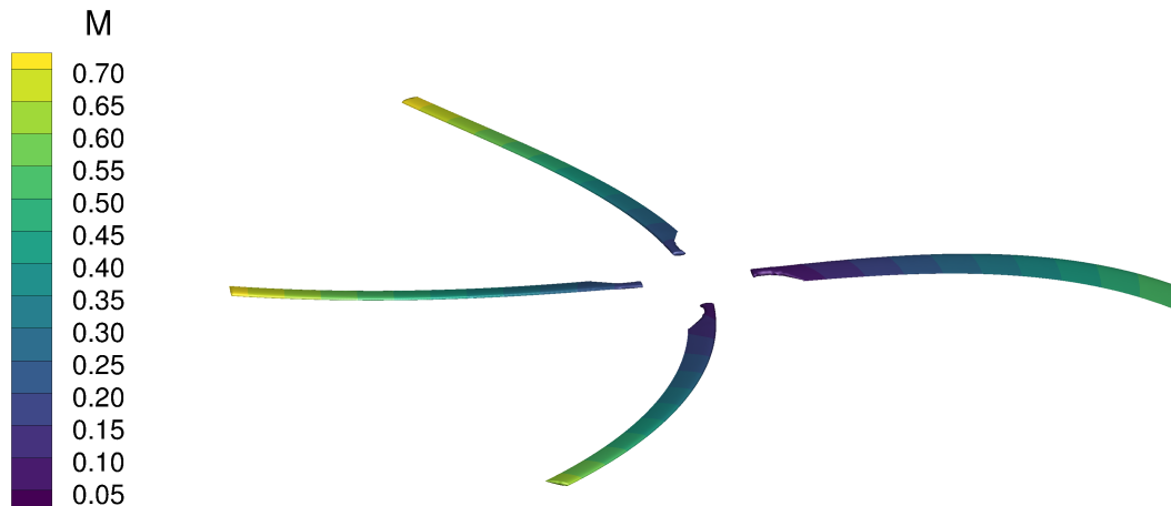
Figure 17: Example metadata output from HART II demonstration case. Isosurface of observer time, colored by Mach number.
