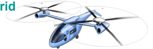
Lift+Cruise Air Taxi Turbo-Electric
