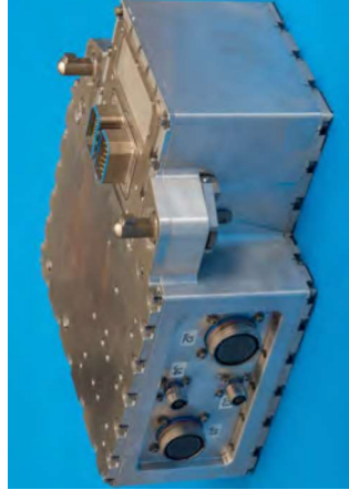
UEI Data Cube and Custom Sensor Supply Printed Circuit Board (Signal Conditioning and Power Distribution)
