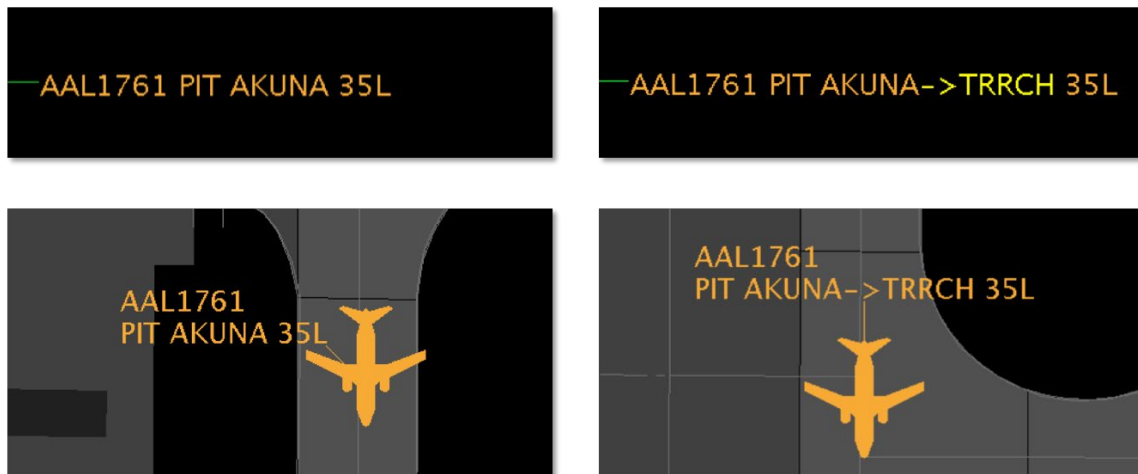
Figure 3.225. Fix Closure Format: Closed Fix (left) and Closed Fix → Alt Fix (right).
