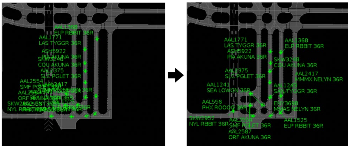
Figure 4.61. Set Up Datablocks: Declutter Tags.
