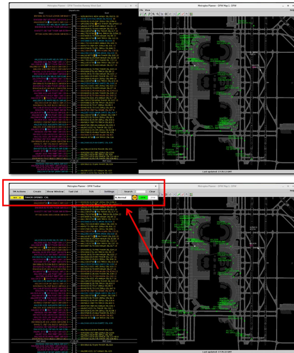
Figure 4.21. Metroplex Planner Toolbar obscured by other windows (top) and displayed in front of other windows (bottom).
