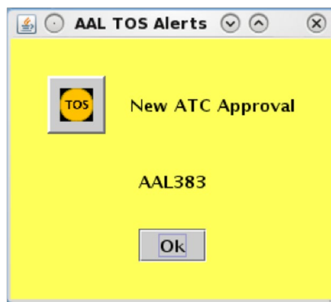
Figure 5.82. TOS Approval pop-up alert in the Flight Operator interface.
