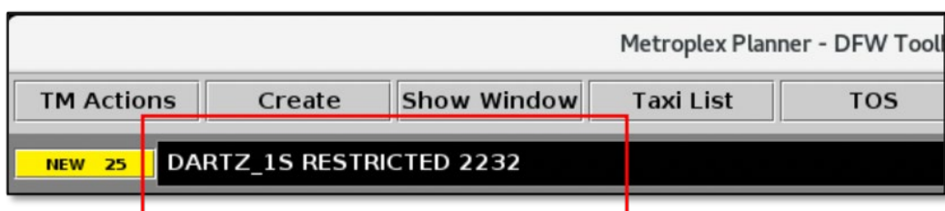
Figure 3.165. Restricted CDR Notification. Start time is shown in hhmm UTC format.
