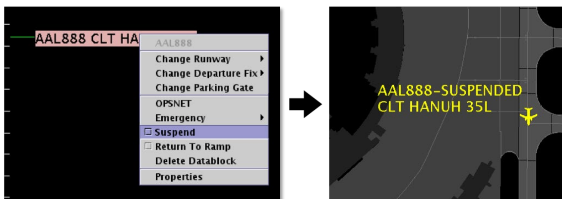
Figure 7.15. Use the right-click menu to select “Suspend” (left). Once selected, the flight is removed from the timeline and “Suspended” is indicated in the flight’s datablock on the map (right).
