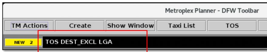
Figure 3.129. Notification: Destination excluded from TOS (in this example, “LGA”).
