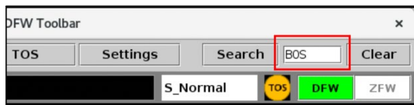
Figure 3.242. Toolbar: Search field (in this example, Destination “BOS” is entered).
