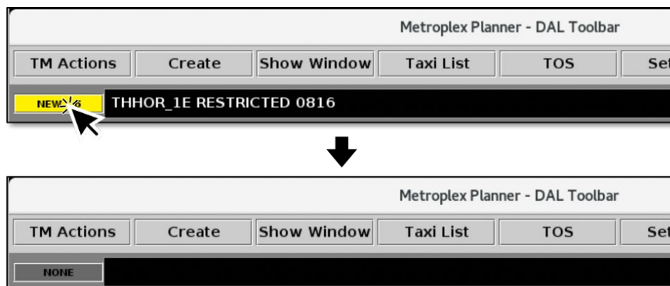
Figure 3.250. Click on the Notification Icon (yellow box) to acknowledge all new notifications.
