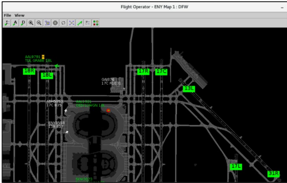
Figure 4.113. Set Up Map: Example of Runway labels on the map.
