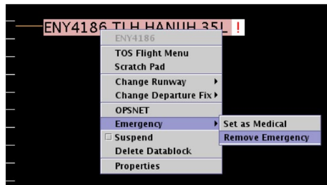
Figure 7.14. Emergency status: Remove Emergency.
