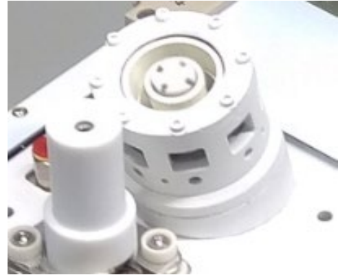
Figure 4.40: ExoMG-nano thruster. Credit: Exotrail.
