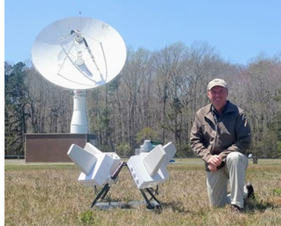
Figure 11.44: ATLAS ground based electrically steered array antenna system. Credit: NASA.
