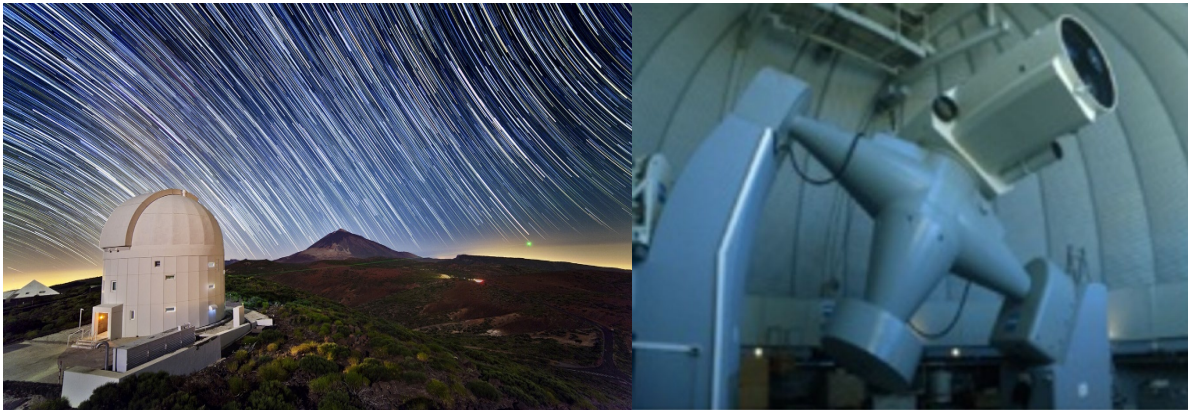
Figure 11.38: (left) ESA-OGS at the Teide Observatory and (right) its 1-meter telescope on an English equatorial mount. Credit: (left) European Space Agency/D. Lopez and (right) European Space Agency.
