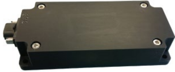
Figure 5.4: NSS Magnetometer. Credit: NewSpace Systems.
