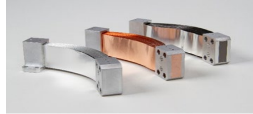
Figure 7.4: Thermal strap design with aluminum foils, copper foils, and PGS in aluminum end blocks (above), and their respective measured thermal conductance (left). The dashed lines connecting data points are based on material thermal conductivity curves. Credit: SDL.
