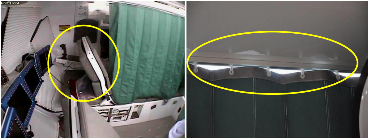
Fig. 11 Interference Concerns and Light Leaks in Rover Cabin Crew Bunk Curtains
