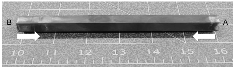
Figure 6.—Photograph showing the direction of the \mu -CT scan from end faces, A and B, of the coated rod up to a distance of 25.4 mm as depicted by the arrows.
