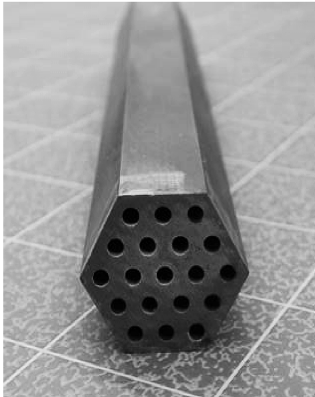
Figure 5.—Photograph of the Mersen 2160 hexagonal rod with 19 channels.
