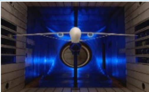
Transonic Truss-Braced Wing 5-10% fuel burn benefit
