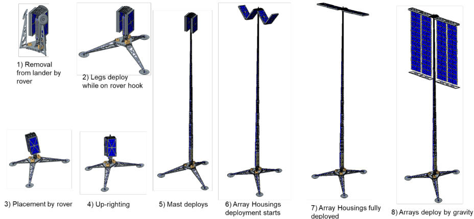
Fig. 5 VSAT Setup and Deployment [5].
