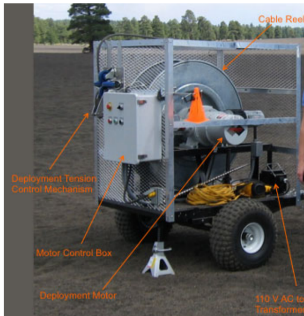
Fig. 8 Prototype Power Cable Deployment Trailer [16].
