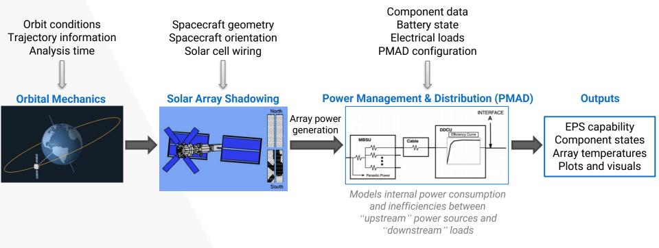
SPACE performs iterative calculations on the EPS model to reach energy balance
