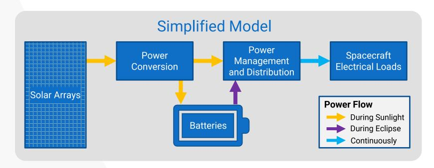
Goal: Ensure spacecraft electrical loads can be powered while maintaining adequate charge in the batteries
