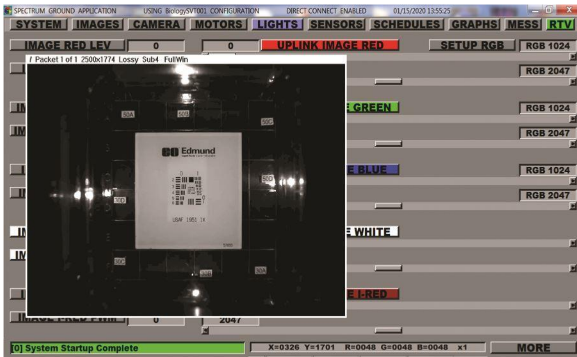
FIGURE 10 – Ground System Application Control Panel showing Real Time View (RTV) in operation over the Image LED Control Panel. RTV uses compression of lower resolution images to support near real time interaction with the SFU during on-orbit operations.
