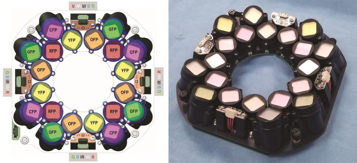
FIGURE 5 – ELS Physical Layout, with CFP, GFP, and RGBW-IR positioned on “outer ring”, axially symmetric about the camera Optic Axis. ELS image is a photograph of the SFU component taken 10 July 2019 during packing for flight.
